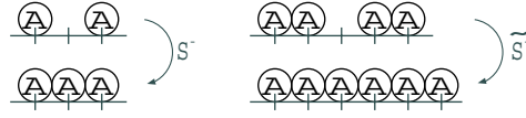
Figure 4. Creation of particles in a monomer and dimer system, yielding ZRP-equivalent states: \tilde{S}^- creates dimers on available and additional volume.
